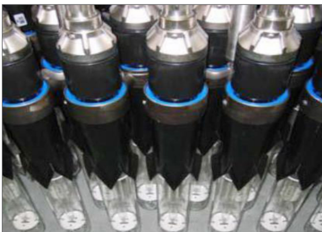
Figure 2: Vortex mixers mounted on quartz sleeves housing medium pressure UV lamps provide additional mixing and direct the low UVT water toward the high intensity light source.
